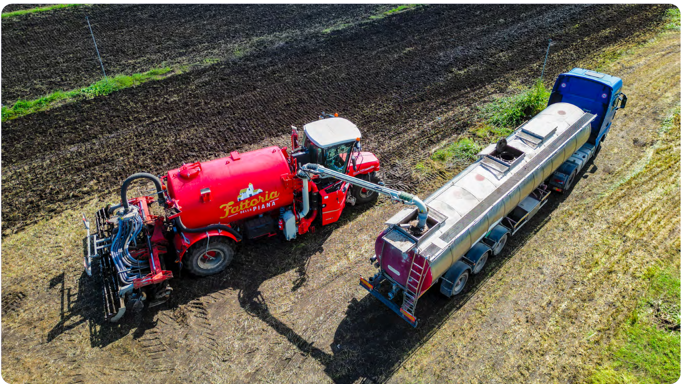
Digestate tanker refuelling the machine used to spread the digestate (Italy).
